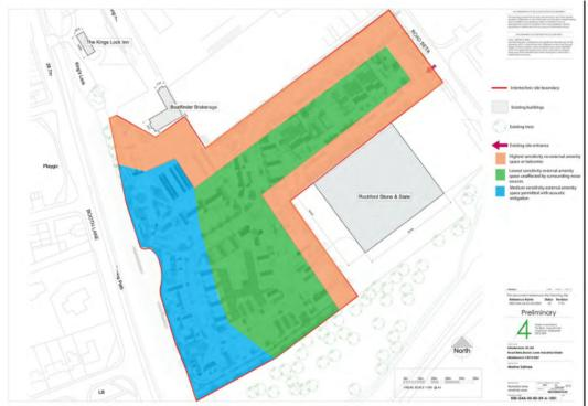
The areas highlighted orange are of the highest sensitivity and should include no external amenity space or balconies. The area highlighted blue are of medium sensitivity external amenity space is permitted with acoustic mitigation. The area highlighted green has the lowest sensitivity external amenity space which is unaffected by surrounding noise sources.
